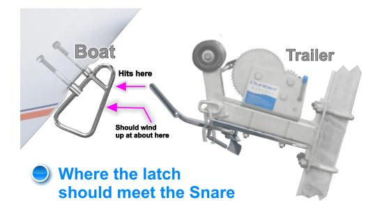
Note the relative positions of the rubber roller/bumper, the point that the snare hits the latch, and the gap between the boat and the rubber roller/bumper.
