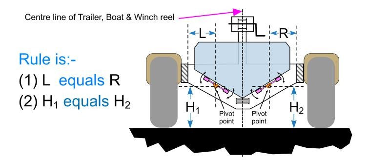
Essentially the boat needs to travel down the centreline of the trailer, with proper support from each side.
