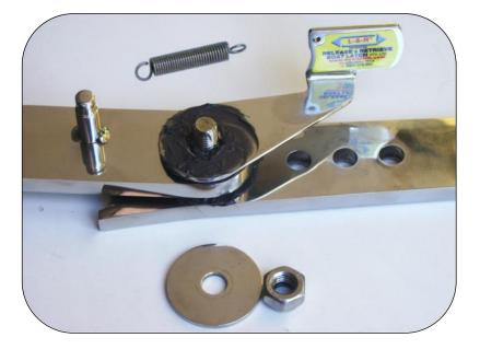
You must grease all contacting parts on assembly. Stainless steel will 'bind' badly if you do not lubricate. Need to use high quality grease (yes that awful black stuff).
